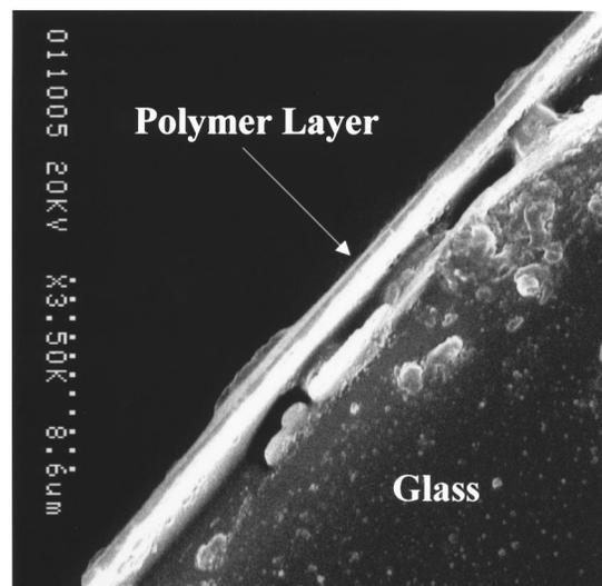
FIG. 3. SEM image showing substrate and polymer film.
