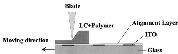
FIG. 1. Schematic illustration of the fabrication process.
